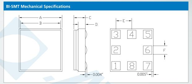
Pad Assignments: Cathode: 1, 3, 5, 7 Anode: 2, 4, 6, 8
