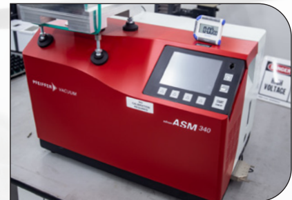
Fine leak testing
