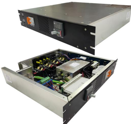
Custom PDUs offer effective and efficient implementation of power distribution, safety features, remote communication, output monitoring, and control.
