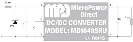
The diagram at left illustrates a simple connection of the MD1000RU series. The TVS provides protection against voltage spikes on the input line. For applications that do not require the circuit to meet EMi/EMC specifications, the capacitors C1 and C2 will reduce input/output ripple and improve the converter stability over time and temperature. The recommended component values are 100 µF for C1 and 10 µF for C2.
