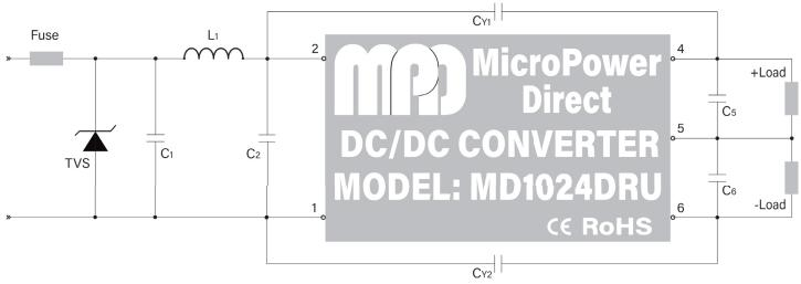
The diagram above shows a typical connection of the MD1000RU series for an application that requires compliance to EMI/EMC standards (as specified on page 1). Some notes on these components are:
