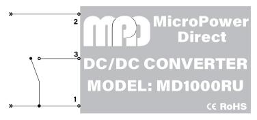
The MD1000RU includes a remote control input. This input (pin 3) is referenced to the minus input (pin 1). The unit operates when this pin is left open, as shown in the diagram at left...
