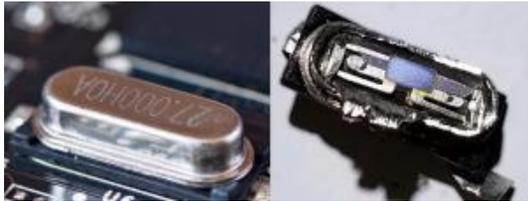
Internals of a Quartz Crystal Oscillator – The quartz crystal is encased in a hermetically sealed package, used as the resonator.
